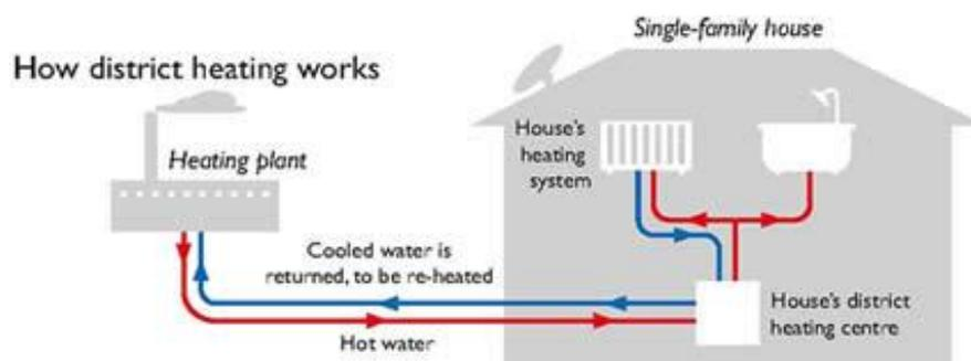
Figure 2 Example of a District Heating system (Source: Linn-Energy.co.uk)
